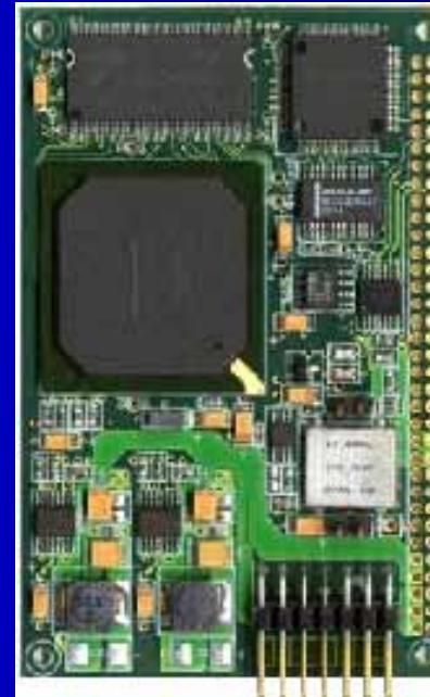
Signal Processor 77 x 51 mm
