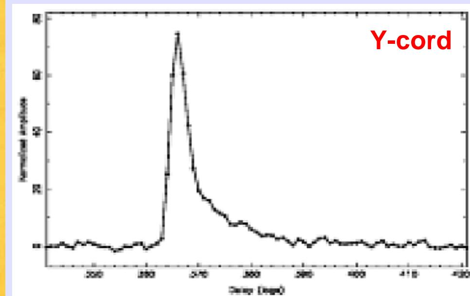
Delay cross-section at zero Doppler
