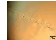
Microscope Image of concentrated defect area
